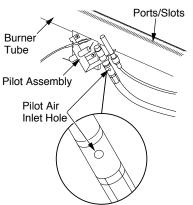
Figure 40 - Pilot Inlet Air Hole
